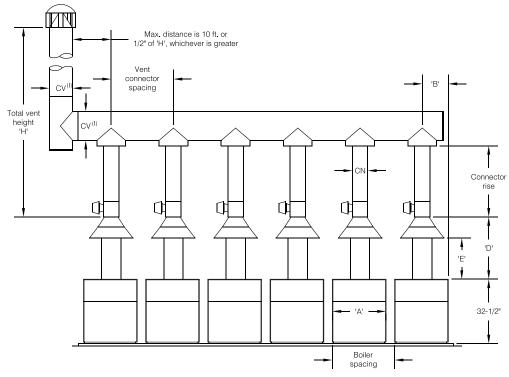
(I) CV based on total boiler input Note: Max. number of boilers venting through CV not to exceed six (6)
