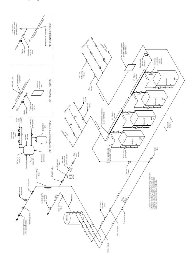
Figure 3-5: Piping Diagram, Primary/Secondary with Pre-Fabricated Manifolds and DHW
