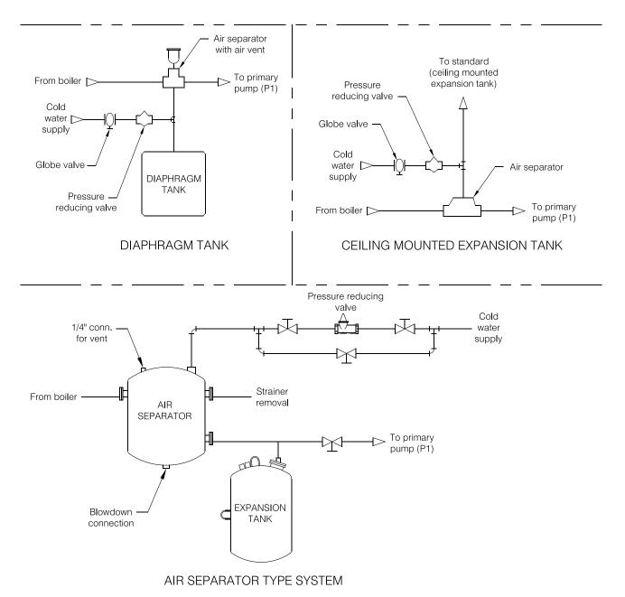
Figure 3-4: Expansion and Air Elimination Details
