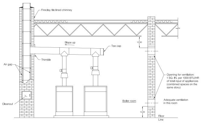
Figure 1-3: Ventilation Air Provided from Inside Building
