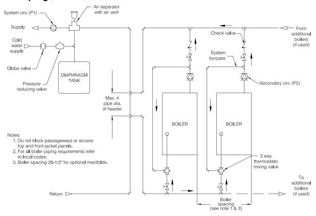
Figure 3-1: Piping Diagram (2 Boilers), Primary/Secondary with Mixing Valves
