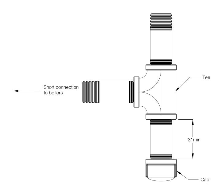
Figure 4-7: Moisture and Dirt Trap for Gas Supply to Each Boiler
