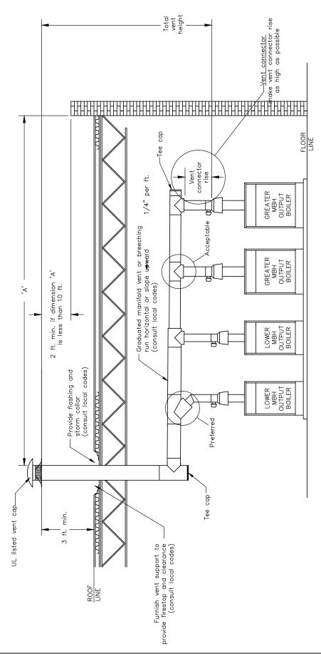
Figure 2-4: Graduated Manifold Vent
