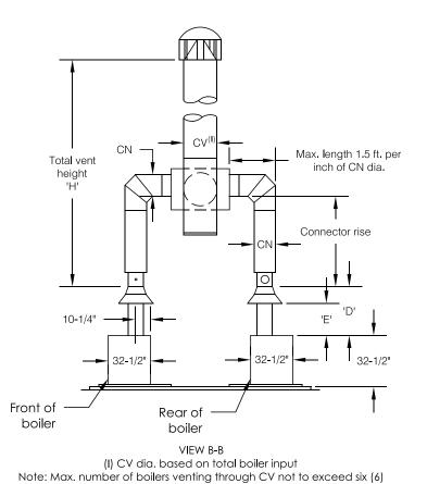
Figure 2-6: Constant Diameter Manifold with Laterals in Vent Connectors
