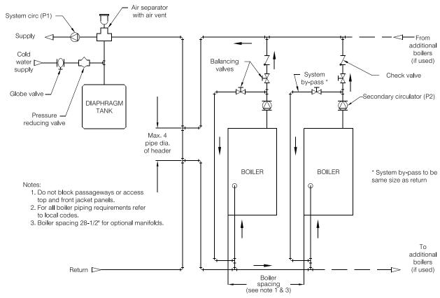
Figure 3-2: Piping Diagram (2 Boilers), Primary/Secondary with By-Pass
