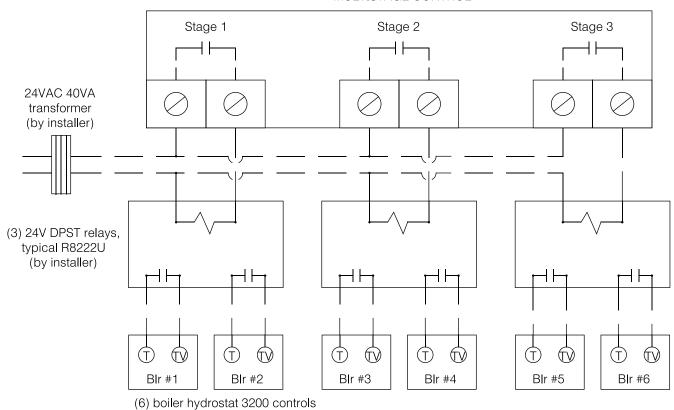
Figure 5-1: Example - Using 24V Relays to Pair Boilers
