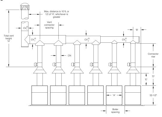
(I) CV, dia. based on total boiler input (6 boilers in this illustration)
