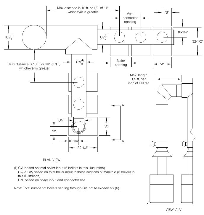
Figure 2-5: Dual Constant Diameter Manifold Vent
