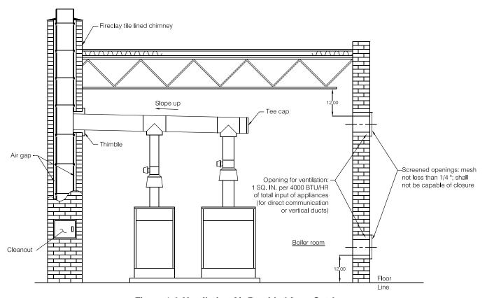
Figure 1-4: Ventilation Air Provided from Outdoors
