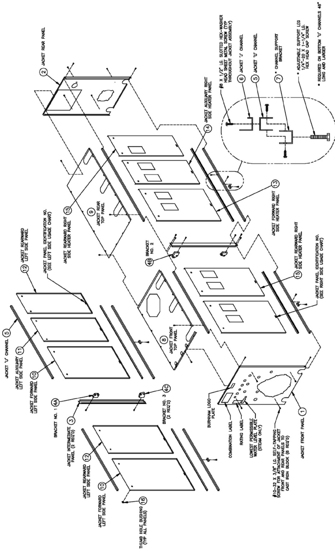
Figure 46: V11H Series Jacket Assembly (Boiler Models V1113H Thru V1123H)
