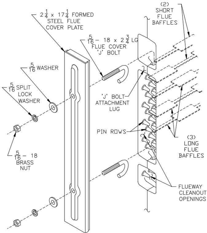
**FLUE BAFFLE AND COVER PLATE INSTALLATION**
