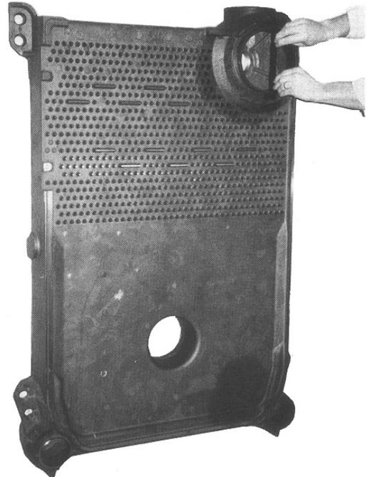
**Figure 6: Setting of Nipples**
