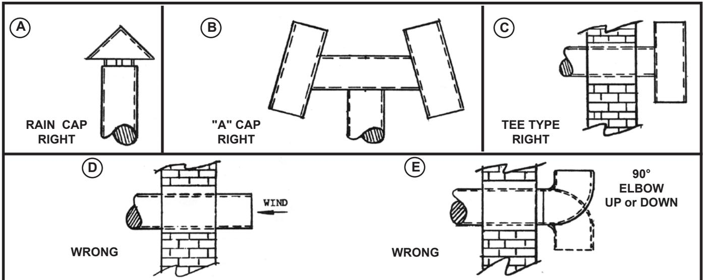
**VENT SIZING** - Area must be the same as or greater than the boiler breeching (Smoke Outlet). A barometric damper may be required on installations with a high draft condition.
