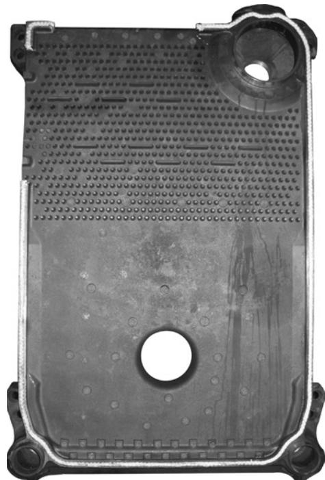
**Figure 7: Affixing the Fiberglass Rope**
