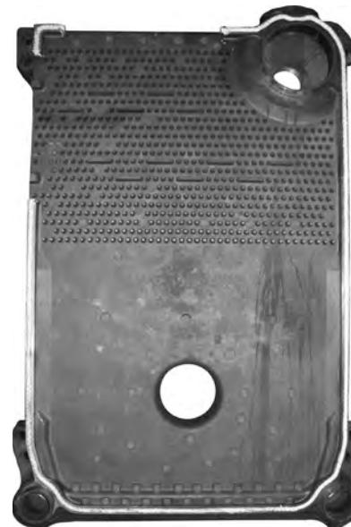
**Figure 7: Affixing the Fiberglass Rope**
