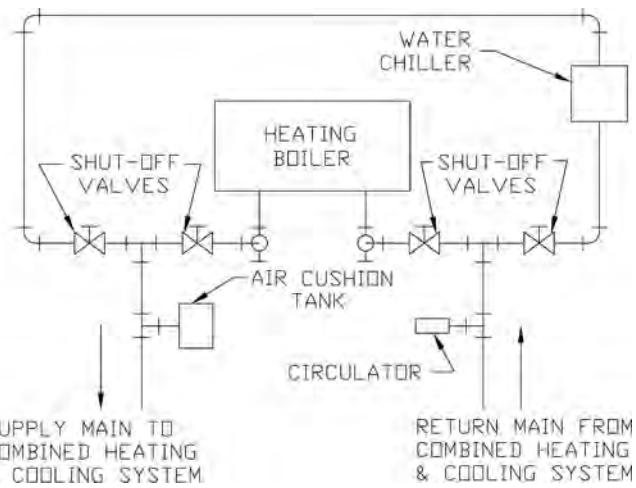
**Figure 40: Recommended Piping for Combination Heating & Cooling (Refrigeration) Systems Water Boilers**
