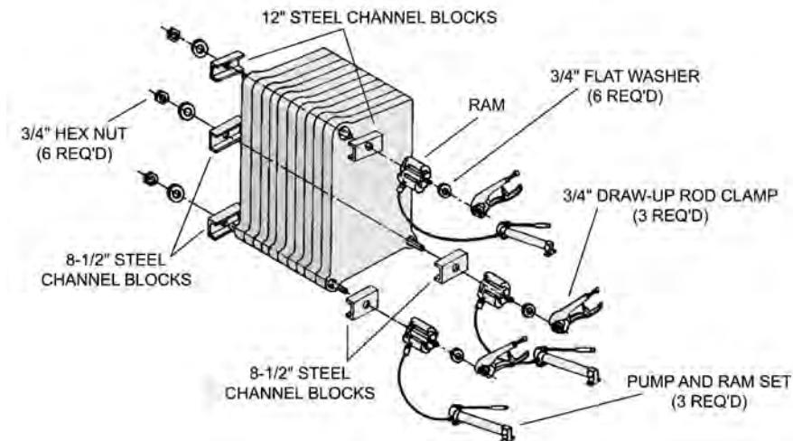
**Figure 13: Hydraulic Draw-Up of Sections**
