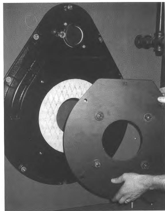
**Figure 26: Burner Mounting Plate and Burner Adapter Plate**
