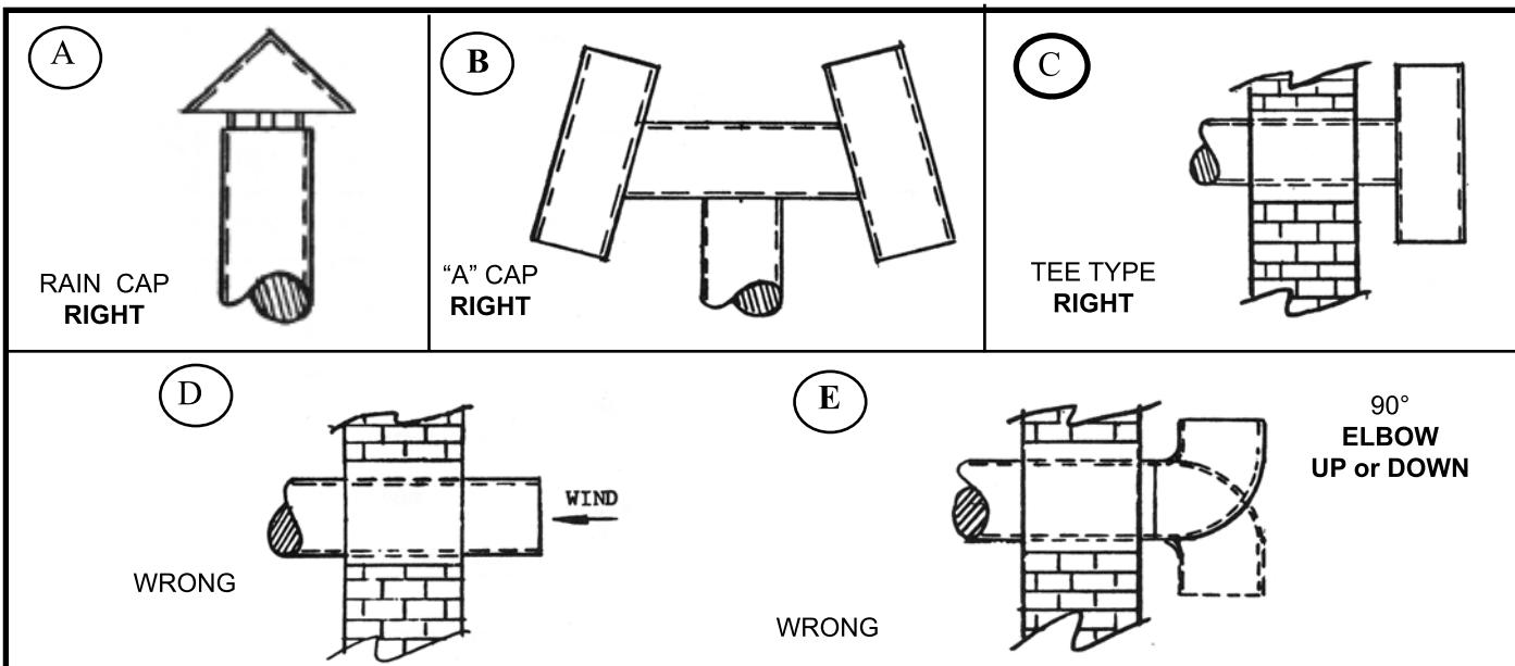
**VENT SIZING** - Area must be the same as or greater than the boiler breeching (Smoke Outlet). A barometric damper may be required on installations with a high draft condition.
