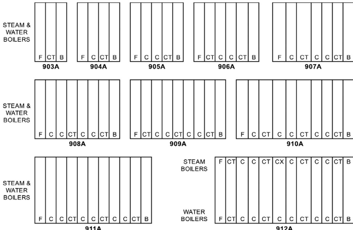
NOTES: FOR BOILERS LESS TANKLESS HEATER, REPLACE THE "CT" SECTIONS WITH "C" SECTIONS. TANKLESS SECTIONS: IF BOILER CAN TAKE MULTIPLE TANKLESS COILS, BUT NOT ALL TANKLESS COILS WILL BE USED, INSTALL COILS TOWARDS BACK OF BOILER, FOLLOWING SECTION ARRANGEMENT CHART.
