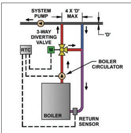
The RTC system is supplied as a kit and can be incorporated into most hydronic hot water applications with minimal modifications to the system design and operation. It provides a simple means for boiler protection and an opportunity to increase operational efficiency.
