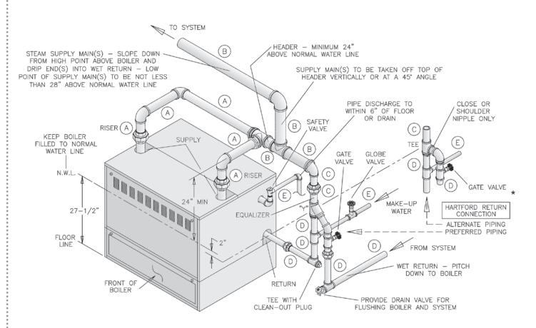
1 or 2 Supply Connections - 5006 thru 5014 \*Required on gravity return systems
