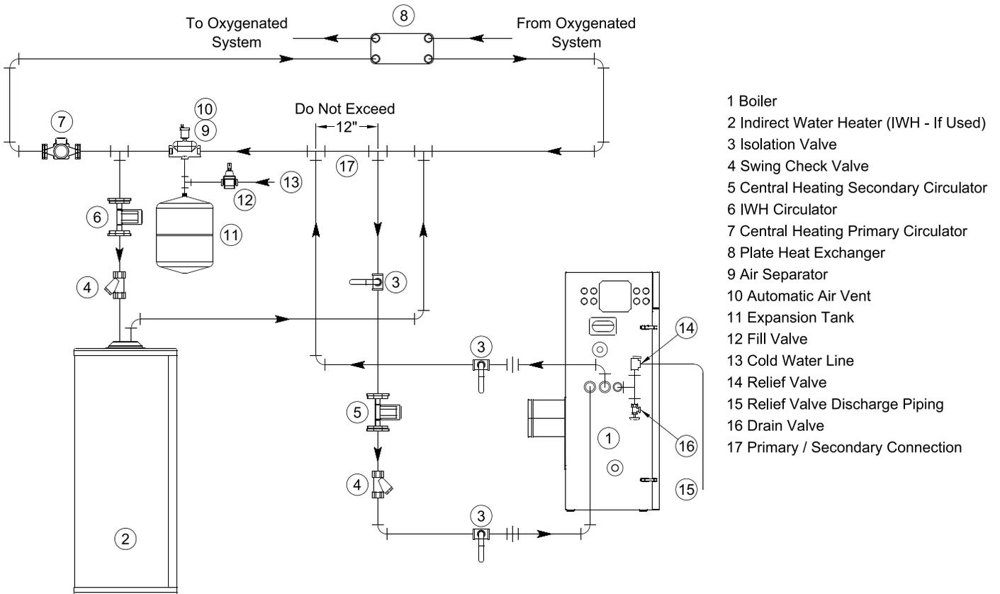
**Figure 38B: Isolation of the Boiler From Oxygenated Water with A Plate Heat Exchanger (IWH Piped Off System Header)**
