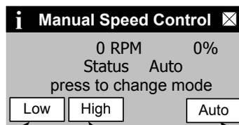
“Press” “Low” to select manual firing rate control and Minimum firing rate %
