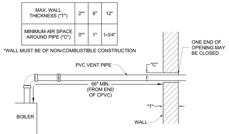
**Figure 8: Wall Penetration Clearances for PVC Vent Pipe**
