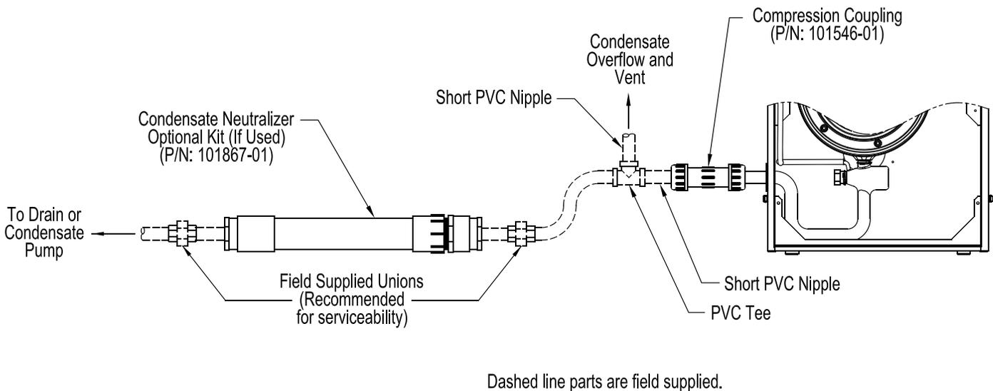
**Figure 34: Condensate Trap and Drain Line**
