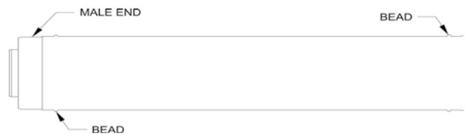
**Figure 19: Fixed Extension (Non-Cuttable)**
