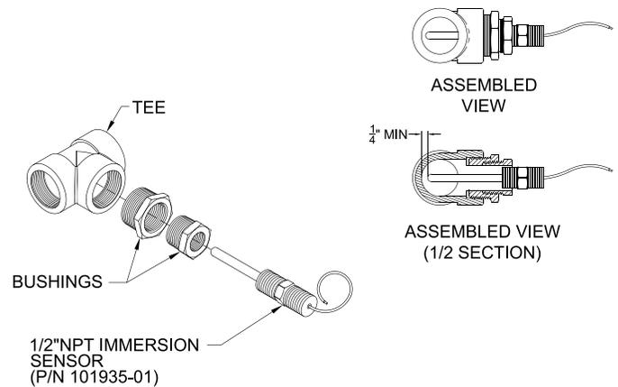
**Figure 48: Recommended Direct Immersion Header Sensor Installation Detail**
