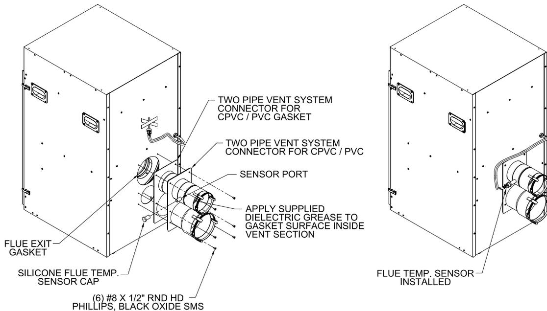
**Figure 6: Field Installation of CPVC/PVC Two-Pipe Vent System Connector**
