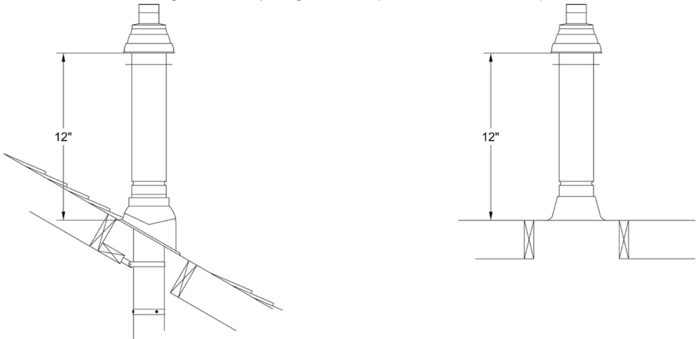
**Figure 27: Vertical Concentric Vent Installation**
