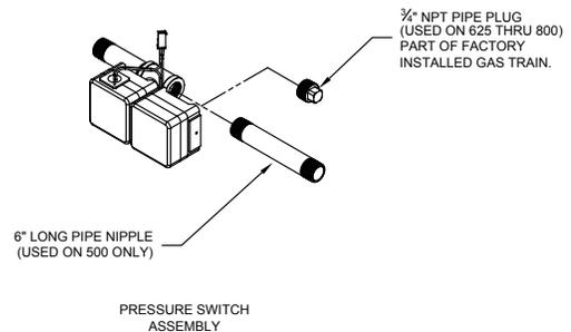
Figure 42: Gas Inlet Pressure Tap and Pressure Switch Location
