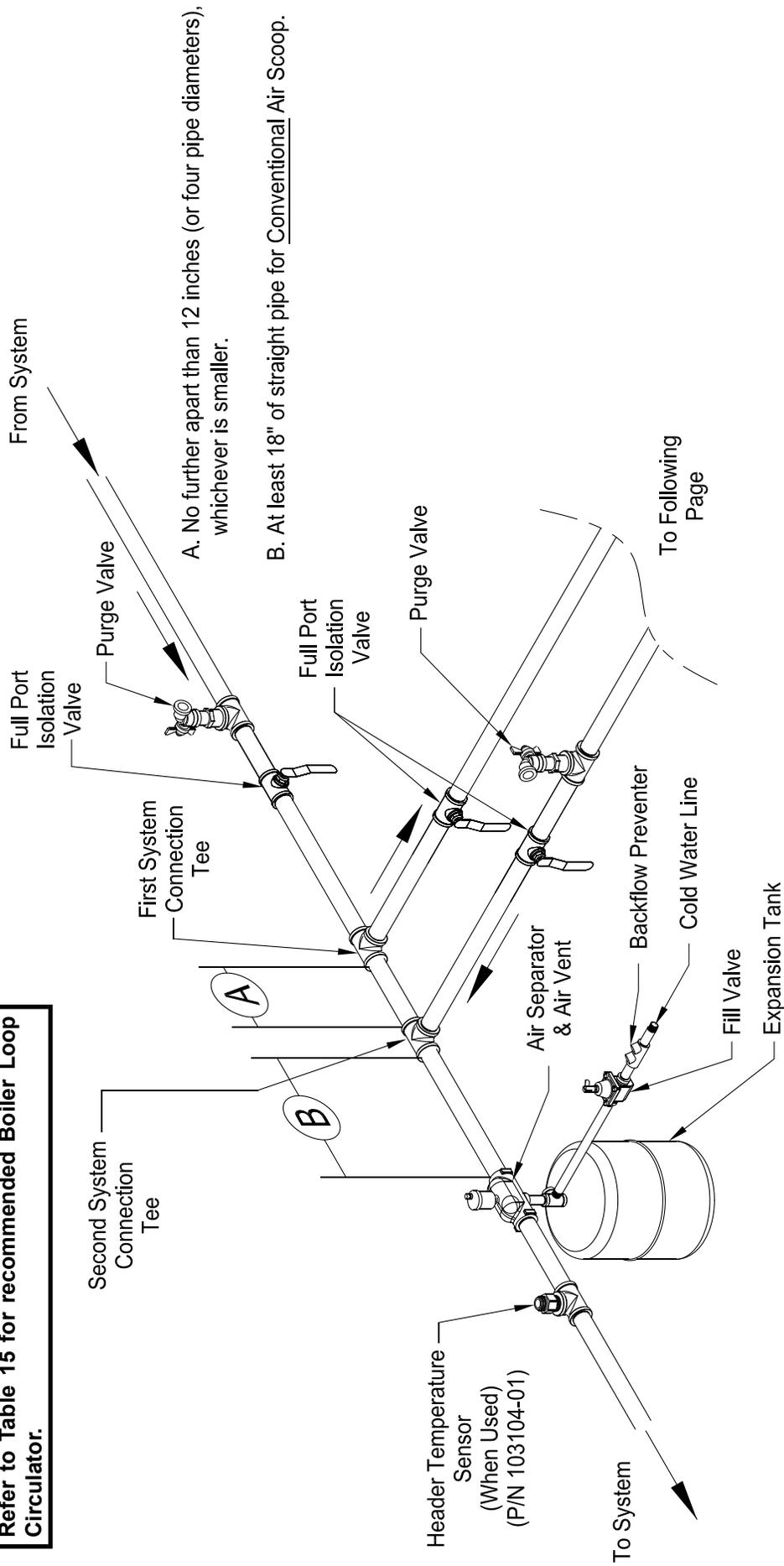
Figure 40A: Alternate Multiple Boiler Water Piping w/ Indirect Domestic Hot Water Heater (Page 1 of 2)
