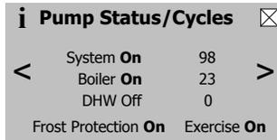
Pumping is a major part of any hydronic system. This screen provides the status of the boiler's demand to connected pumps as well as the status of Frost Protection and pump Exercise functions.
