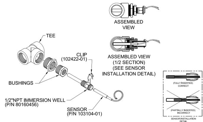
**Figure 49: Alternate “Immersion” type Header Sensor Installation Detail**
