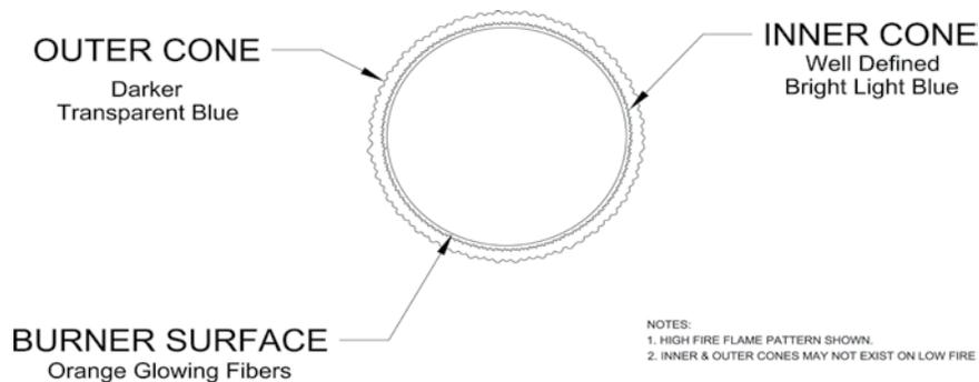
**Figure 52: Burner Flame**
