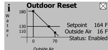
Outdoor Reset saves energy and improves home comfort by adjusting boiler water temperature. This screen presents the active reset curve. The curve shows the relationship between outside air and outdoor reset setpoint. The curve shown is adjustable by entering the display's adjust mode.
