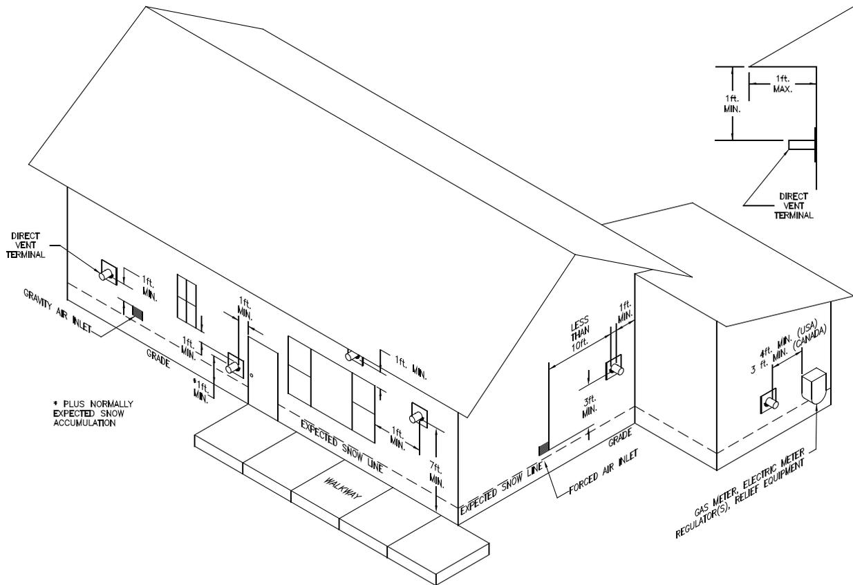
**Figure 4: Location of Vent Terminal Relative to Windows, Doors, Grades, Overhangs, Meters and Forced Air Inlets
