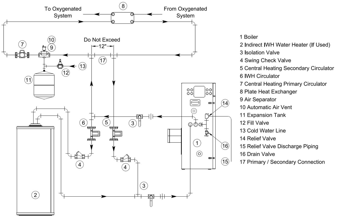
**Figure 38A: Isolation of the Boiler From Oxygenated Water with A Plate Heat Exchanger (IWH Piped as Part of Boiler Piping)**
