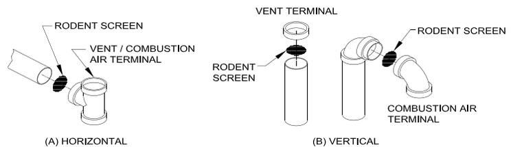
**Figure 10: Rodent Screen Installation**
