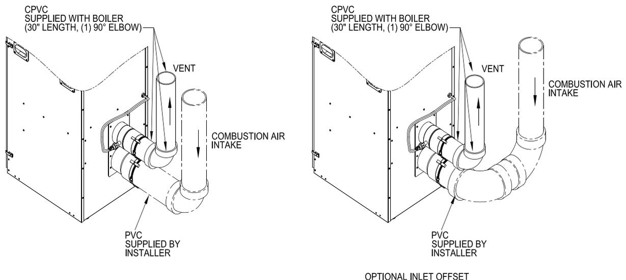
**Figure 7: Near-Boiler Vent/Combustion Air Piping**
