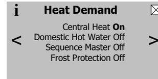
This screen provides the status of the boiler's 4 possible heat demands. When demand is off the Control has not detected the call-for-heat.
